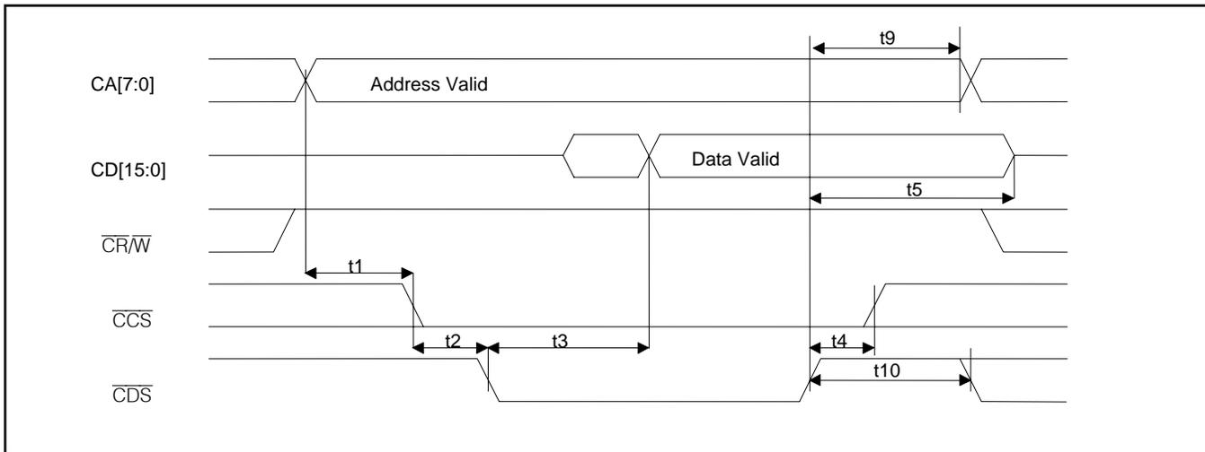
**Figure 13-7. Motorola Write Cycle (Nonmultiplexed)**
