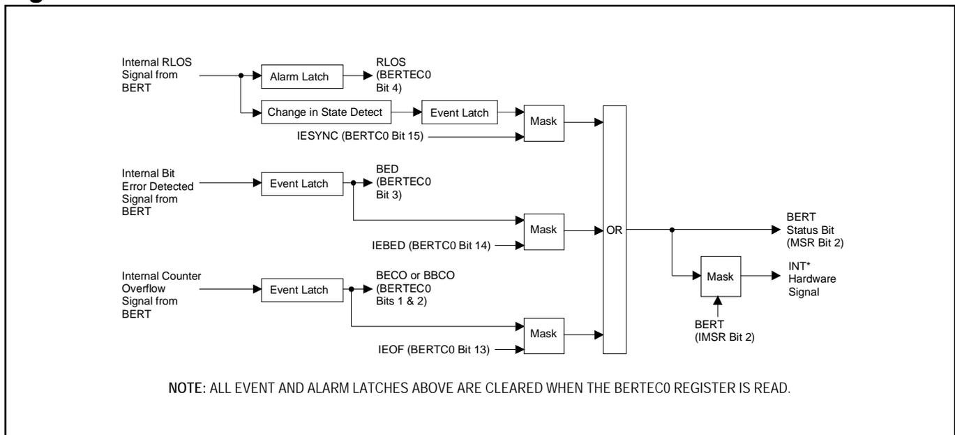
**Figure 4-5. HDLC Status Bit Flow**
