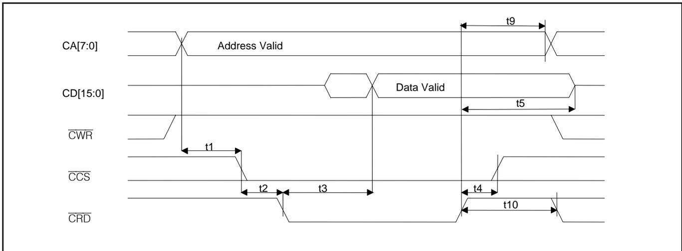
**Figure 13-5. Intel Write Cycle (Nonmultiplexed)**
