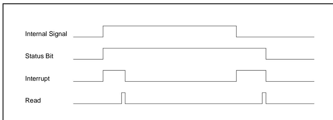
**Figure 4-3. Real-Time Status Bit**
