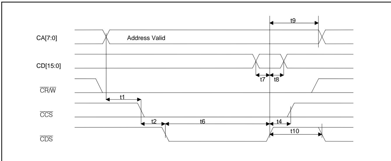
**Figure 13-8. Intel Read Cycle (Multiplexed)**
