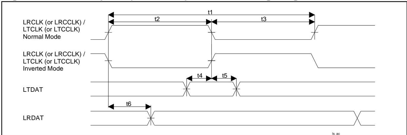
**Table 13-2. AC Characteristics—High-Speed (T3 and E3) Ports**
