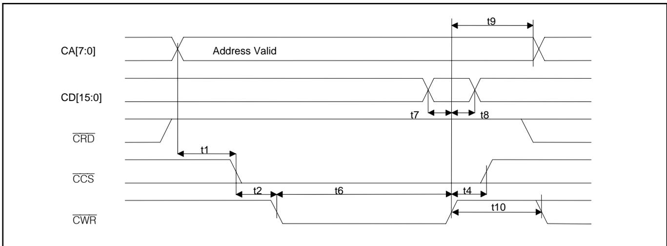
**Figure 13-6. Motorola Read Cycle (Nonmultiplexed)**
