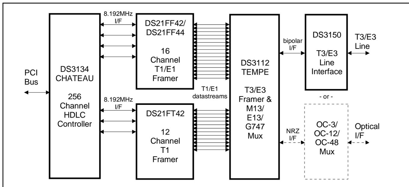
**Figure 14-2. Unchannelized Dual T3/E3 Application**
