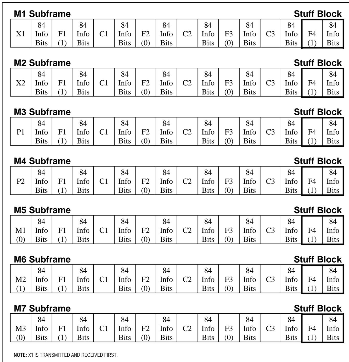
**Figure 14-6. T3 Stuff Block Structure**
