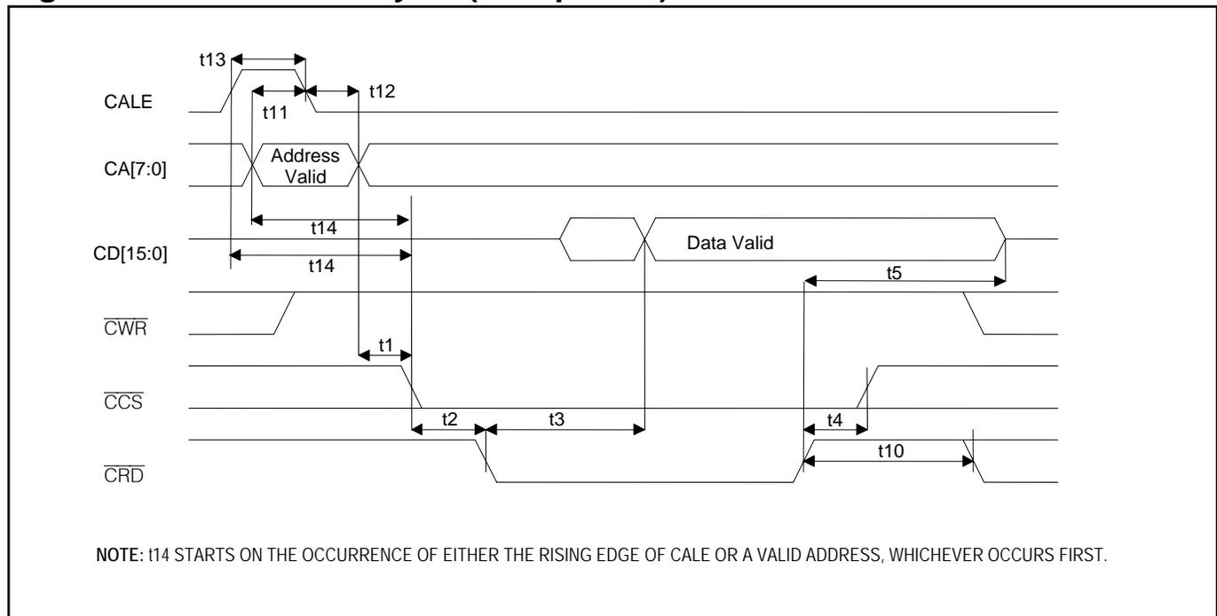
**Figure 13-9. Intel Write Cycle (Multiplexed)**
