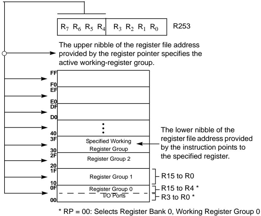
**Figure 14. Register Pointer—Detail**
