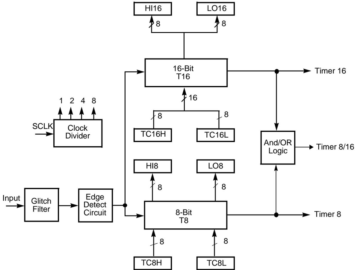
Figure 2. Counter/Timers Diagram
