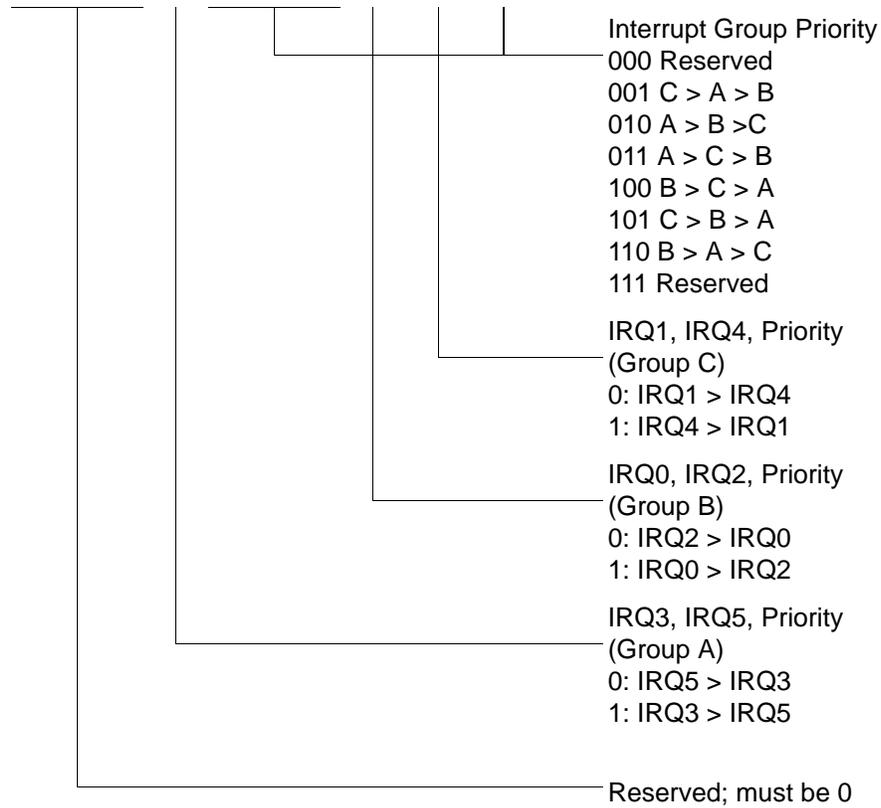
**Figure 48. Interrupt Priority Register (F9H: Write Only)**
