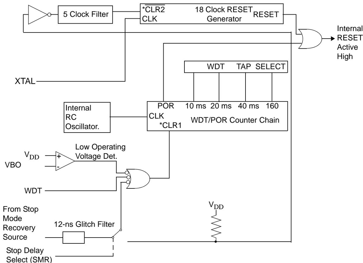
\* CLR1 and CLR2 enable the WDT/POR and 18 Clock Reset timers respectively upon a Low-to-High input translation.
