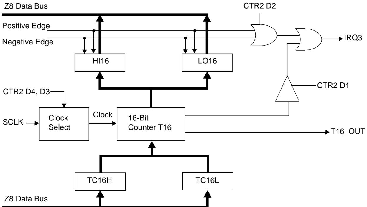
**Figure 22.16-16-Bit Counter/Timer Circuits**
