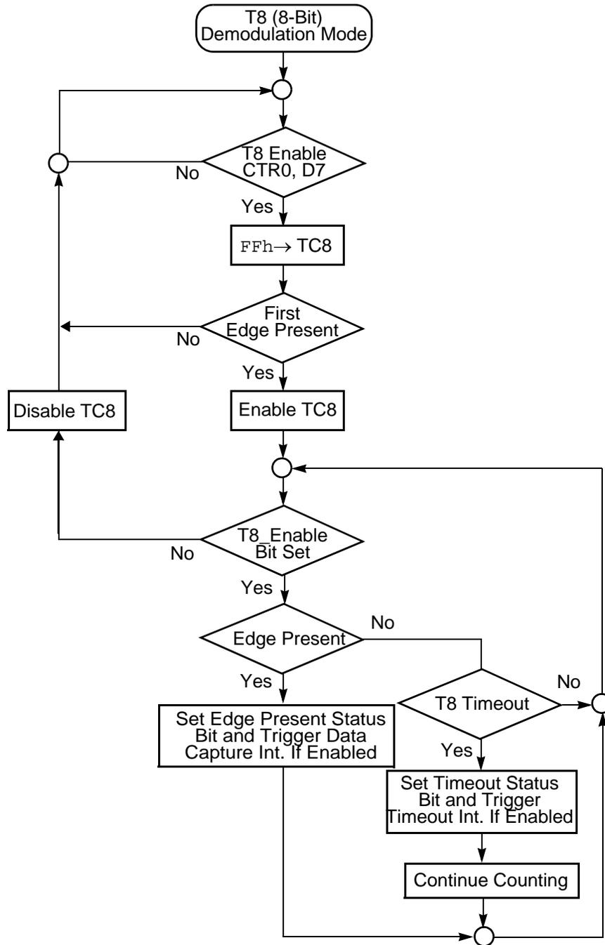
Figure 21. DEMODULATION Mode Flowchart
