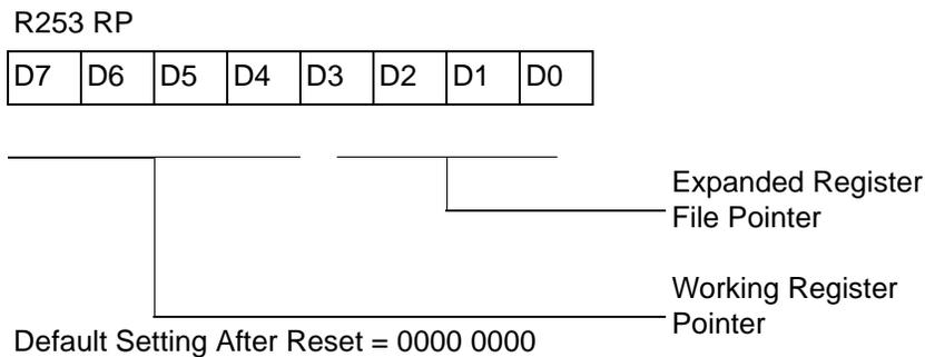
**Figure 13. Register Pointer**
