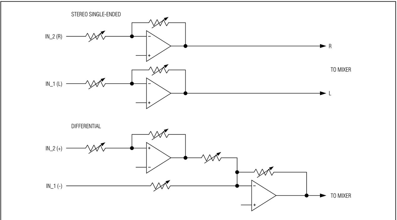
Figure 2. Differential and Stereo Single-Ended Input Configurations
