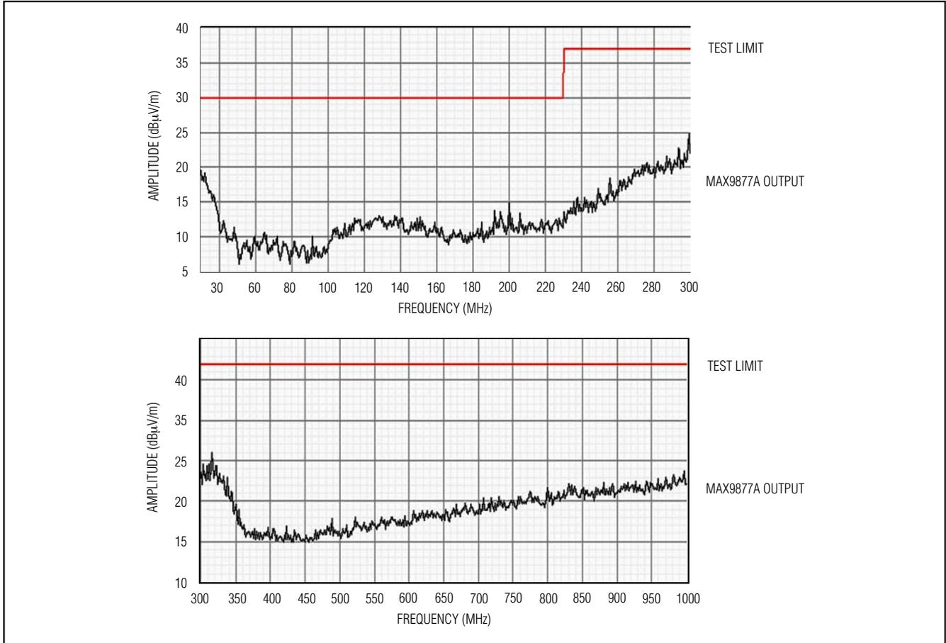
Figure 4. EMI with 152mm of Speaker Cable
