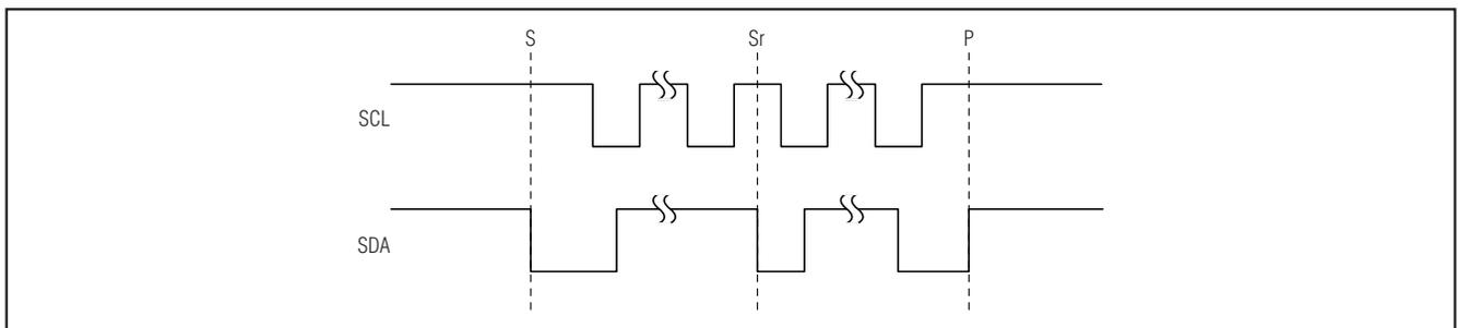
Figure 7. START, STOP, and REPEATED START Conditions
