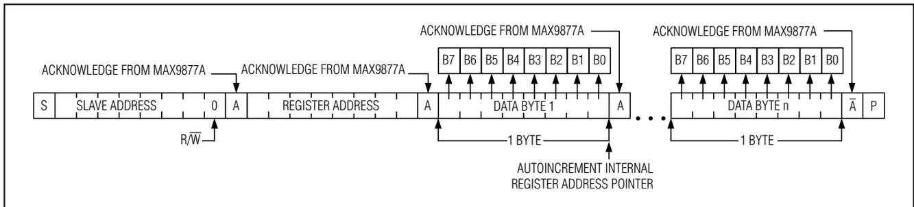
Figure 10. Writing n-Bytes of Data to the MAX9877A
