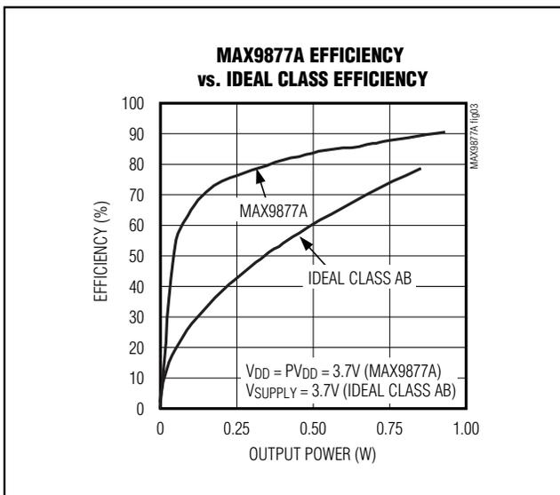
Figure 3. MAX9877A Efficiency vs. Class AB Efficiency
