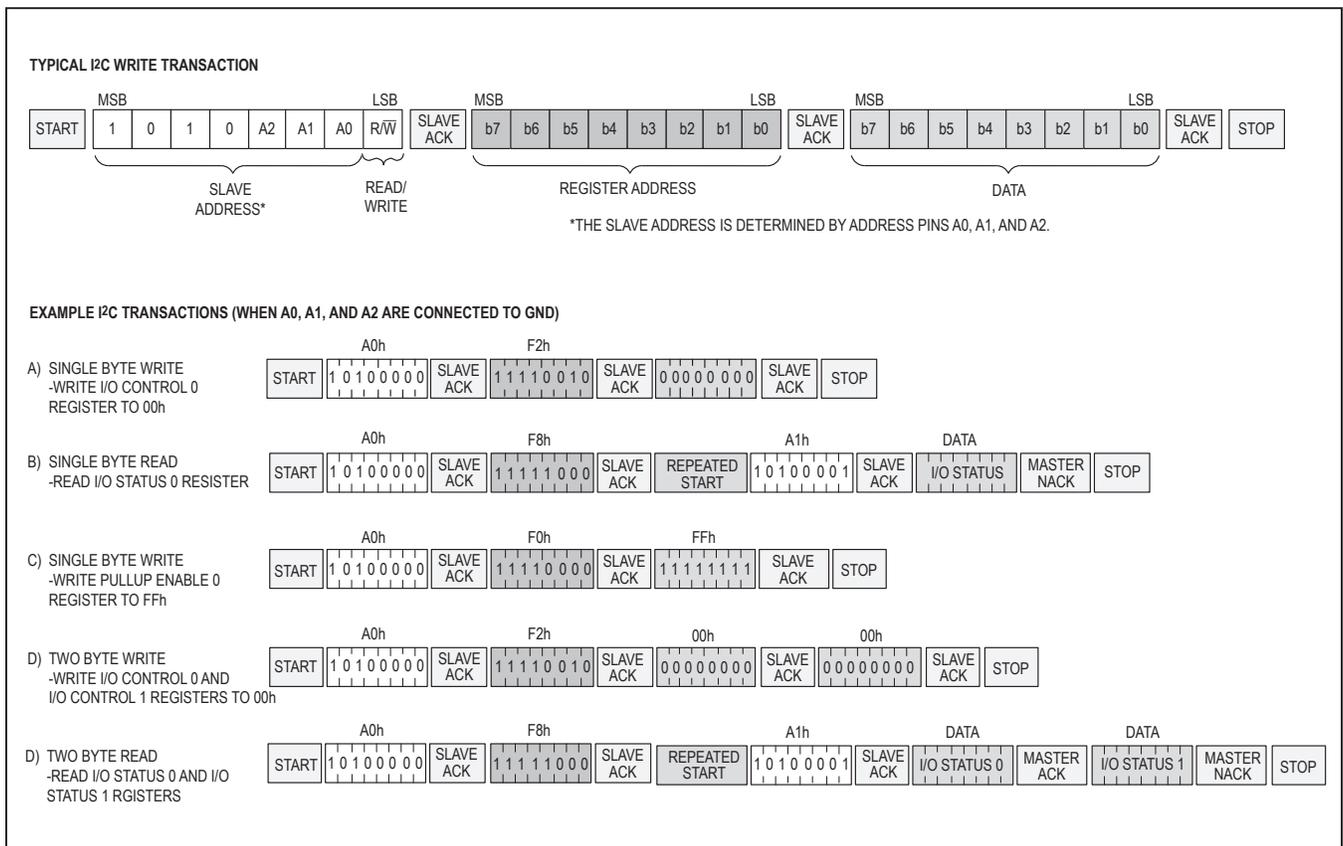
Figure 6. I<sup>2</sup>C Communication Examples
