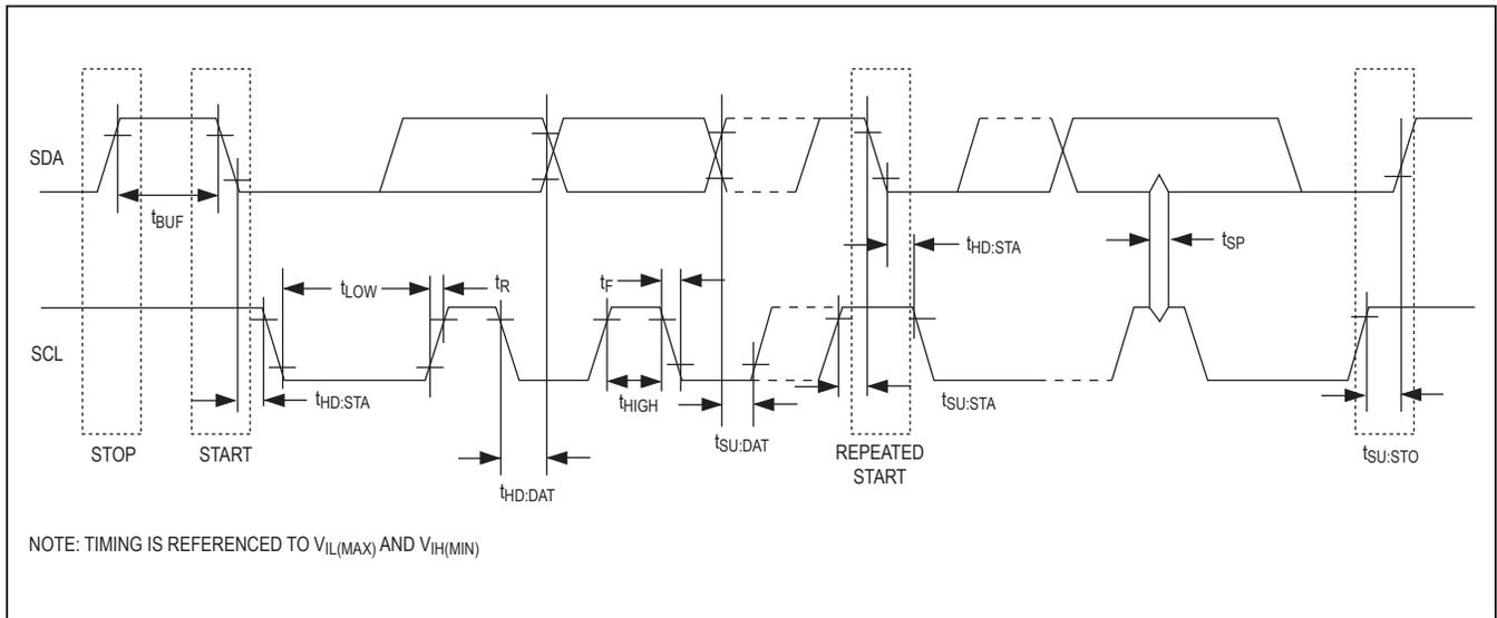
Figure 5. I<sup>2</sup>C Timing Diagram
