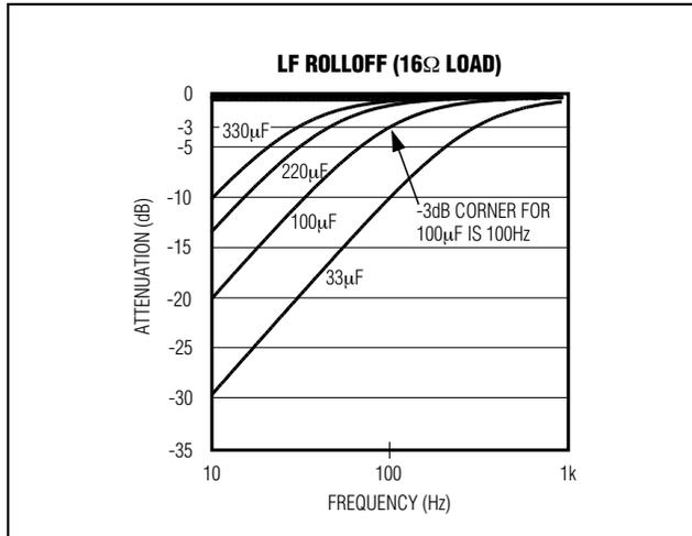
Figure 2. Low-Frequency Attenuation for Common DC-Blocking Capacitor Values
