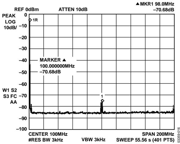
Figure 4.  $F_{OUT} = 1 \text{ MHz}$ ,  $F_{CLK} = 400 \text{ MSPS}$ , WBSFDR
