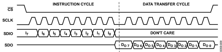
Figure 22. 3-Wire Serial Port Read Timing—Clock Stall Low
