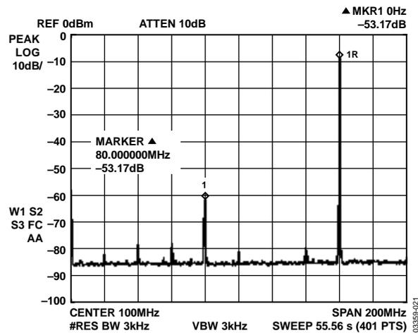
Figure 9.  $F_{OUT} = 160 \text{ MHz}$ ,  $F_{CLK} = 400 \text{ MSPS}$ , WBSFDR
