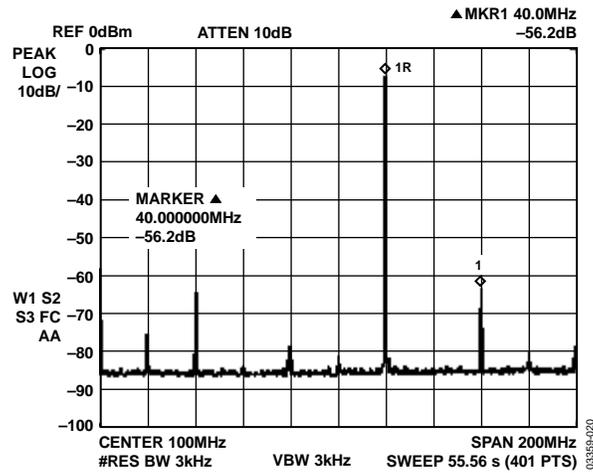
Figure 8.  $F_{OUT} = 120 \text{ MHz}$ ,  $F_{CLK} = 400 \text{ MSPS}$ , WBSFDR
