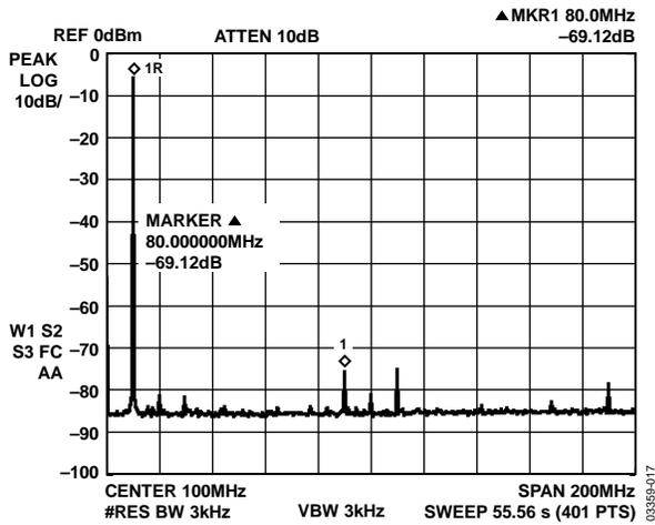
Figure 5.  $F_{OUT} = 10 \text{ MHz}$ ,  $F_{CLK} = 400 \text{ MSPS}$ , WBSFDR
