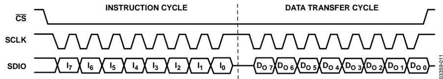
Figure 24. 2-Wire Serial Port Read Timing—Clock Stall High
