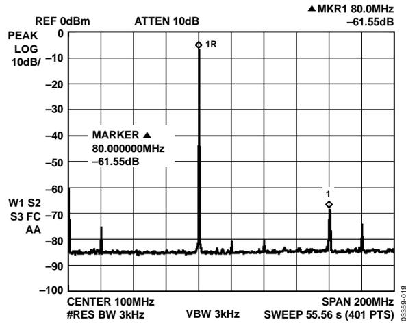
Figure 7.  $F_{OUT} = 80 \text{ MHz}$ ,  $F_{CLK} = 400 \text{ MSPS}$ , WBSFDR
