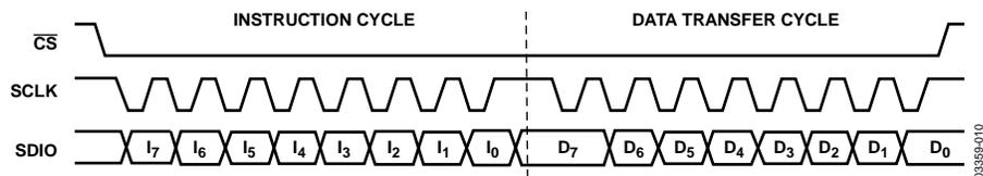
Figure 23. Serial Port Write Timing—Clock Stall High
