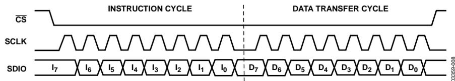
Figure 21. Serial Port Write Timing—Clock Stall Low
