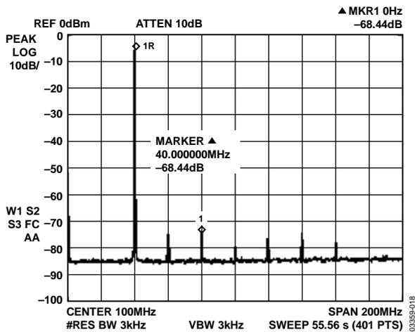
Figure 6.  $F_{OUT} = 40 \text{ MHz}$ ,  $F_{CLK} = 400 \text{ MSPS}$ , WBSFDR
