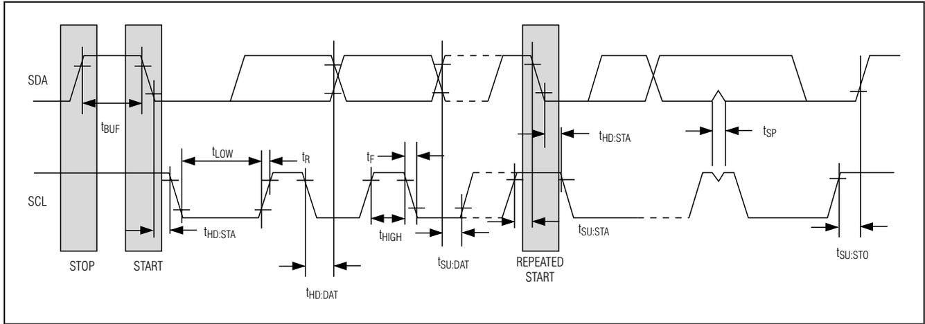
Figure 4. Data Transfer on I<sup>2</sup>C Serial Bus
