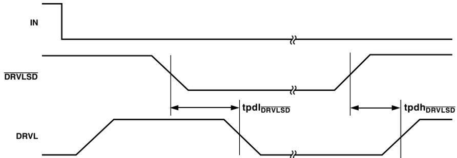
Figure 3.  $\overline{\text{DRVLS}}$  Propagation Delay
