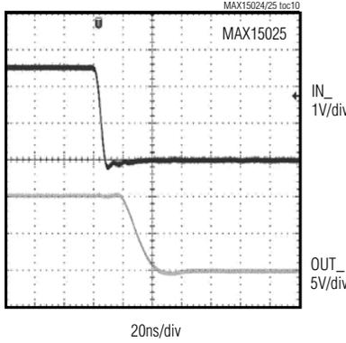
**LOGIC INPUT VOLTAGE vs. OUTPUT VOLTAGE
