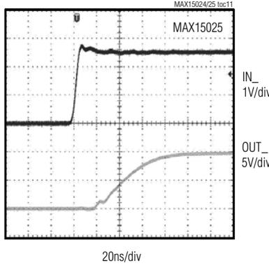
**LOGIC INPUT VOLTAGE vs. OUTPUT VOLTAGE
