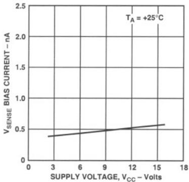
Figure 17. ADP3811  $V_{SENSE}$  Bias Current vs.  $V_{CC}$
