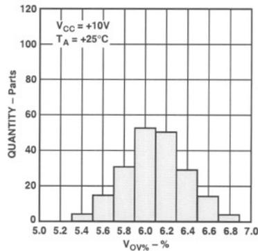
Figure 18. Overtolerance Comparator Distribution ( $V_{OV\%}$ )
