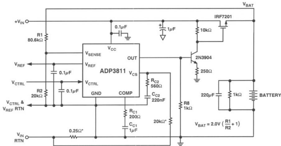
Figure 29. ADP3811 Controlling a Linear Battery Charger
