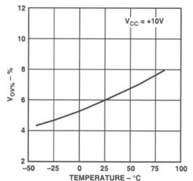
Figure 19. Overtolerance Comparator Threshold ( $V_{OV\%}$ ) vs. Temperature
