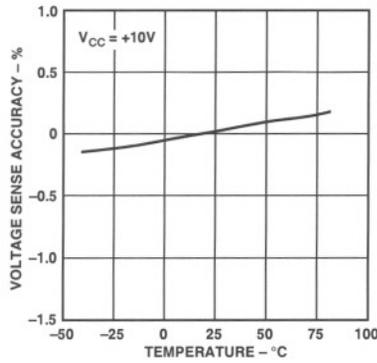
Figure 12. ADP3810 Voltage Sense Accuracy vs. Temperature
