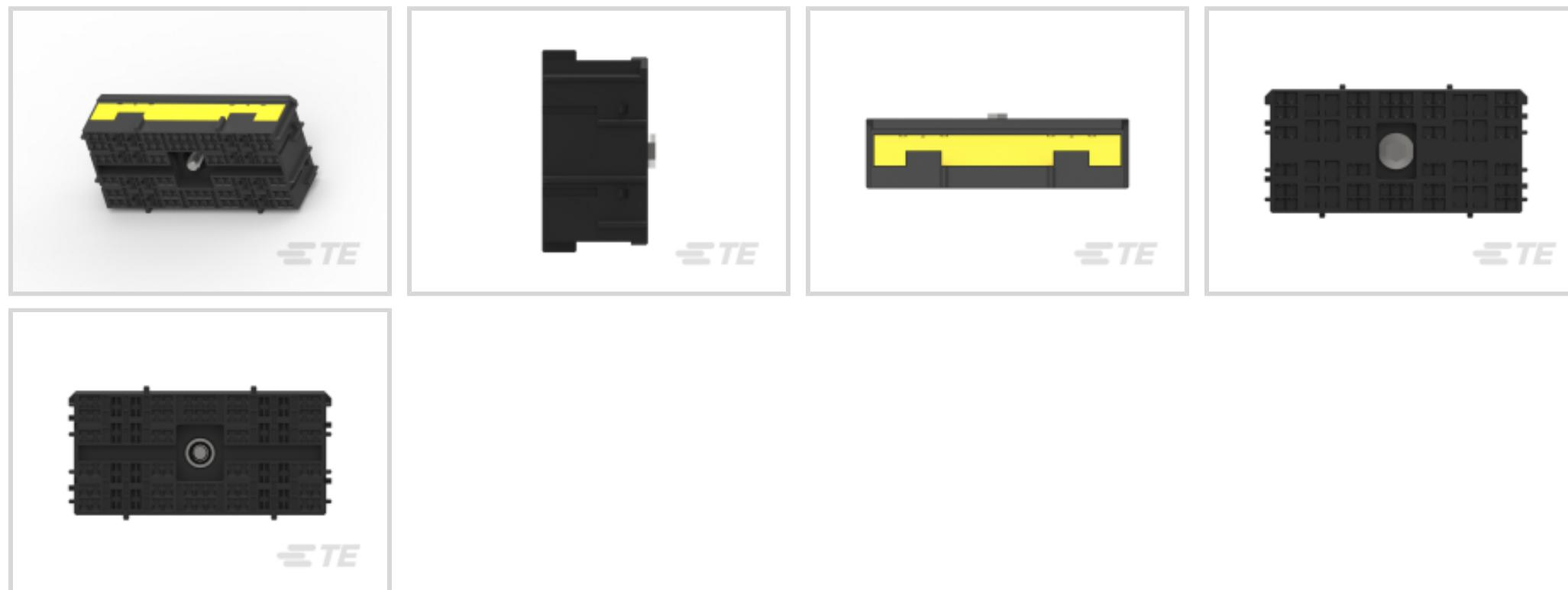
Connector System: **Wire-to-Wire**Number of Positions: **76**Connector & Housing Type: **Housing for Female Terminals**Sealable: **No**Mating Tab Width: **6.3 mm [.248 in]**[All MULTILOCK, CONNECTOR HOUSING \(567\)](#)**Features****Product Type Features**
