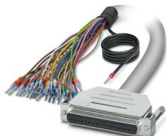
Assembled shielded round cable; connection 1: Single wires (37-position) (The wires are marked and fitted with ferrules. The braided shield is routed to a separate cable end.); connection 2: D-SUB socket strip (1x 37-position); cable length: 10 m
