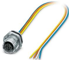
Device connector, rear mounting, PROFINET CAT5 (IEC 11801:2002), 4-position, Socket, straight, M12-Push-Pull, coding: D, on free cable end, Rear mounting, M16 x 1.5, Individual wires, cable length: 0.5 m, 0.34 mm<sup>2</sup>, TPE litz wire, Alternative product in accordance with RoHS II without Exemption 6c (Pb <0.1%) item no.: 1238101
