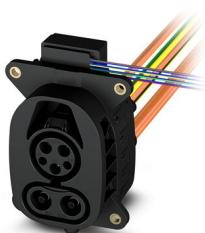
CHARX connect universal, Vehicle charging inlet, for charging with alternating current (AC) and with direct current (DC), CCS type 1, IEC 62196-2, IEC 62196-3, 200 A / 1000 V (DC), 48 A / 250 V (AC), Single wires, length: 2 m, locking actuator: 12 V, 4-pos., Front and rear mounting, M6, housing: black, A protective cap is supplied as standard for the DC and AC contacts.
