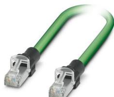
Patch cable, degree of protection: IP20, cable length: 5 m, number of positions: 4, 100 Mbps, CAT5, material: PP, connection method: Pierce connection, connection cross section: AWG 23-22, cable outlet: straight, PROFINET
