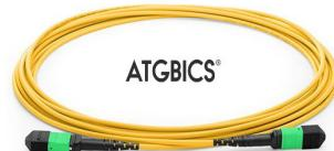
ATGBICS MPO Female-Female 12 Fibres OS2 9/125 Singlemode Trunk Cable, Type B, LSZH 3.0, 1m
