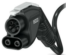
CHARX connect compact, DC charging cable, with vehicle charging connector and open cable end, for charging electric vehicles (EV) with direct current (DC), with connected CS contact, with analog temperature sensors, CCS type 1, SAE J1772, IEC 62196-3, 80 A / 1000 V (DC), PHOENIX CONTACT logo, cable: 4 m, black, straight
