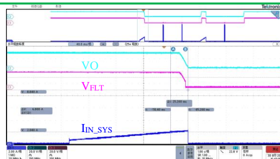
Overload Performance with MX26631DL during Load Step from 0A to 3A
