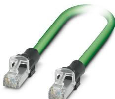
Patch cable, degree of protection: IP20, cable length: 15 m, number of positions: 4, 100 Mbps, CAT5, material: PP, connection method: Pierce connection, cable outlet: straight, PROFINET
