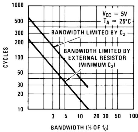
Figure 5-9. Greatest Number of Cycles Before Output
