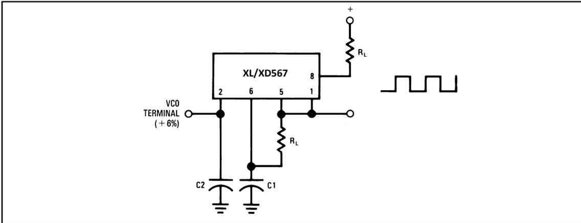
Figure 8-7. Precision Oscillator Drive 100-mA Loads
