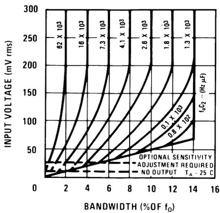
Figure 5-5. Bandwidth vs Input Signal Amplitude
