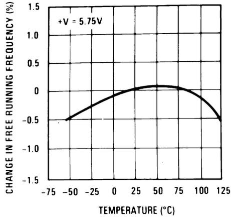
Figure 5-1. Typical Frequency Drift
