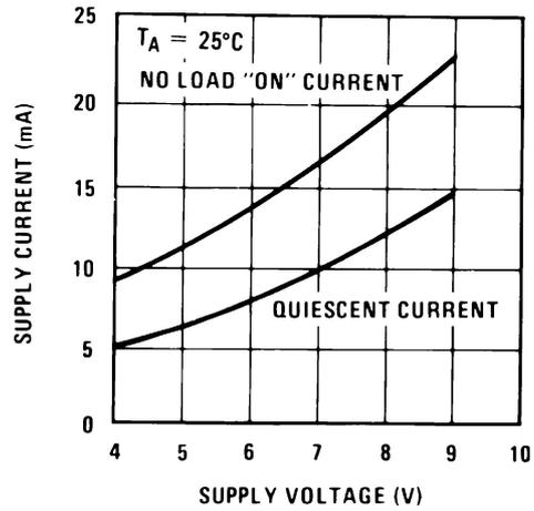
Figure 5-8. Typical Supply Current vs. Supply Voltage
