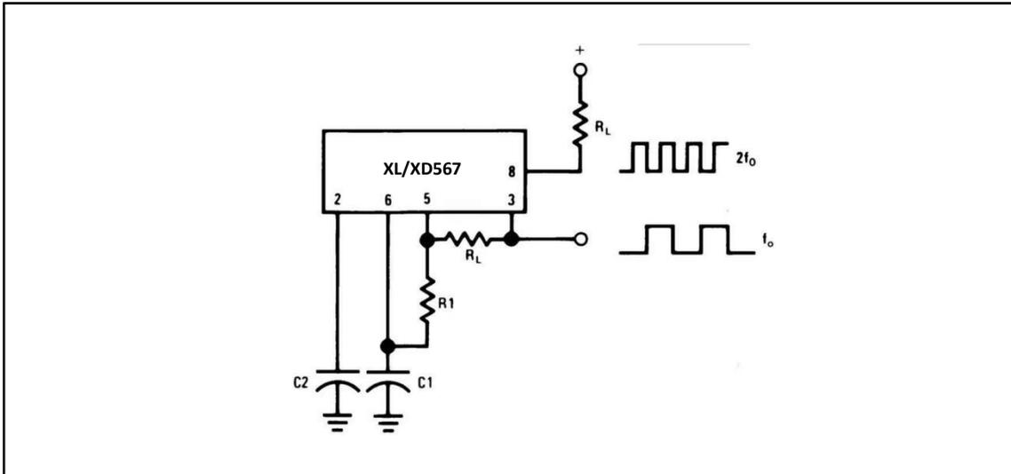
Figure 8-5. Oscillator with Double Frequency Output
