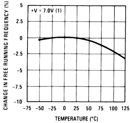
Figure 5-4. Typical Frequency Drift
