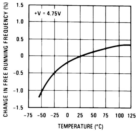
Figure 5-3. Typical Frequency Drift
