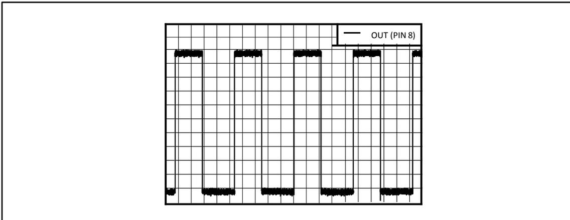
Figure 10-8. Output for 100-mA Load
