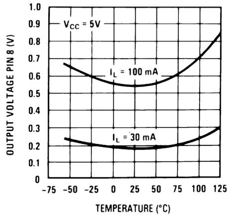
Figure 5-10. Typical Output Voltage vs. Temperature
