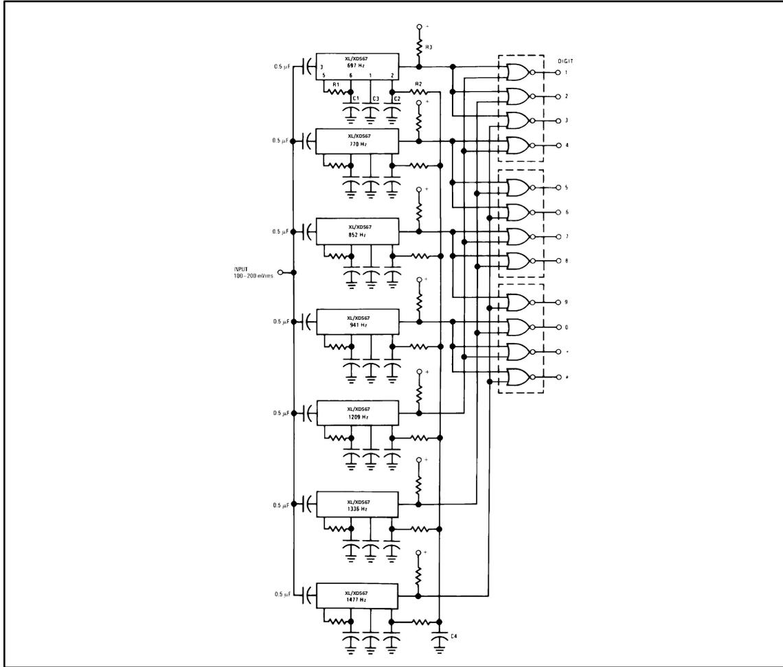
Component values (typ) R1 6.8 to 15k R2 4.7k R3 20k C1 0.10 mfd C2 1.0 mfd 6V C3 2.2 mfd 6V C4 250 mfd 6V
