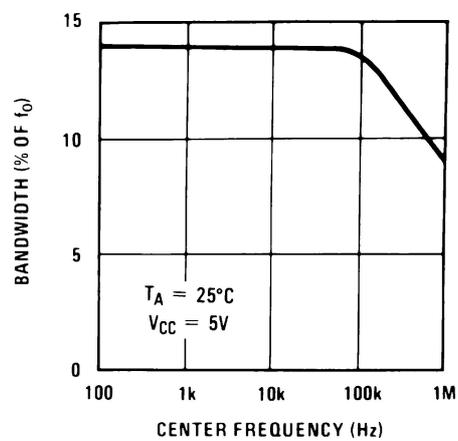
Figure 5-6. Largest Detection Bandwidth
