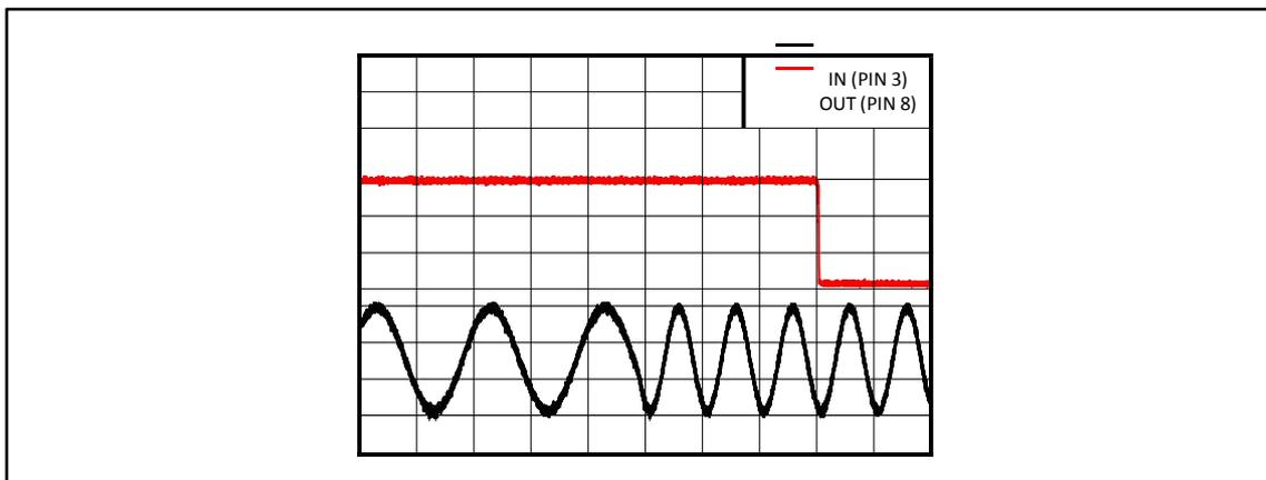
Figure 8-2. Frequency Detection
