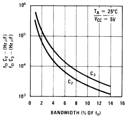
Figure 5-7. Detection Bandwidth as a Function of  $C_2$  and  $C_3$  vs
