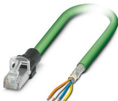
Patch cable, degree of protection: IP20, cable length: 1 m, number of positions: 4, 100 Mbps, CAT5, material: PP, connection method: Pierce connection, connection cross section: AWG 23-22, cable outlet: straight, PROFINET
