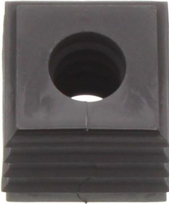
Seal, Mounting type: Plug in, Length x width: 20.3 mm, Max. cable diameter: 10 mm, IP 66, Colour: Black
