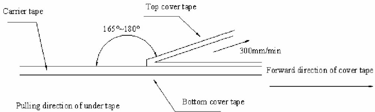
\*\*\* In the case, the cover tape is pulled off under the above conditions, the cover tape adhesion strength should be 10.2g~71.4g
