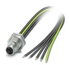
Device connector, rear mounting, Power, 5-position, straight, M12, coding: K M12, Rear mounting, M16 x 1.5, Individual wires, cable length: 0.5 m, 2.50 mm², PEX litz wire, Alternative product in accordance with RoHS II without Exemption 6c (Pb <0.1%) item no.: 1238537
