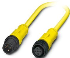
Sensor/actuator cable, 4-position, TPE, yellow, Plug straight M12, coding: A, on Socket straight M12, coding: A, cable length: 12 m
