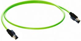
Fast Ethernet Cat5e Data Double-Ended Cordset: Male straight RJ45-coded black RJ45 Field Attachable to male straight RJ45-coded black RJ45 Field Attachable, shielded, 30 V AC / 42 V DC, 1.5 A; TPE green cable, 4-wires, 0.38 mm<sup>2</sup>
