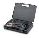
HCS assembly kit for SC-RJ quick mounting connectors, including stripping blade, stripping pliers, aramide yarn scissors, fiber stripper, microscope, fiber cleaving tool for standard HCS and HCS GI fibers, two SC-RJ connectors for standard HCS fiber, and documentation
