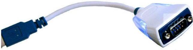
The Cable incorporates a standard USB-A device connector for connection to an upstream host or hub port. RS232-level signals, including modem handshake signals, are available on an industry-standard DE-9P connector. The maximum RS232-level data rate is 1MBaud.
