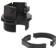
Split cable gland including counter nut, Thread type: metric, Material: PA 6.6, Protection: IP 66, Colour: Black
