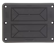
Cable entry flange plate with foamed-in frame gasket, Mounting type: Screw, Length: 165 mm, Width: 123 mm, IP66, Colour: Black
