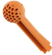
Using the KDS BW1 actuating tool, the seals can be conveniently mounted in and dismantled from the frame. The ergonomic grip and the special shape enable simple and precise installations, especially for cabling applications in confined spaces., Material: Polyamide
