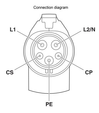
Pin assignment of the Vehicle Connector
