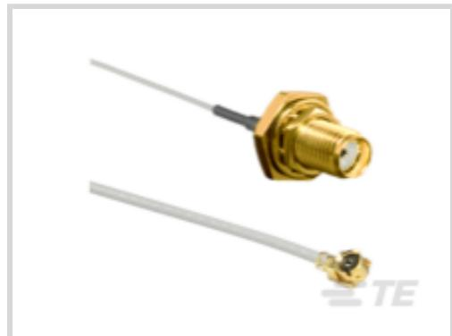
Connector Type (End A): **SMA Jack**Cable Assembly Length: **.15 m [ .492 ft ]**Connector Type (End B): **UMCC Plug**Impedance: **50 Ω**Operating Frequency: **6 GHz**
