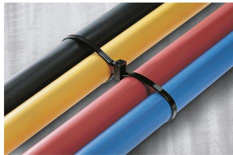
The tie contains a dual locking design to secure two bundles at once. Head design can also provide spacing between parallel bundles. Bent tail allows for quick insertion into head.
