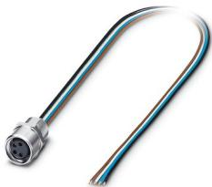
Device connector front mounting, 4-position, Socket, straight, M8, Front mounting, M8 x 0.5, Individual wires, cable length: 2.5 m, 0.25 mm<sup>2</sup>, PVC litz wire
