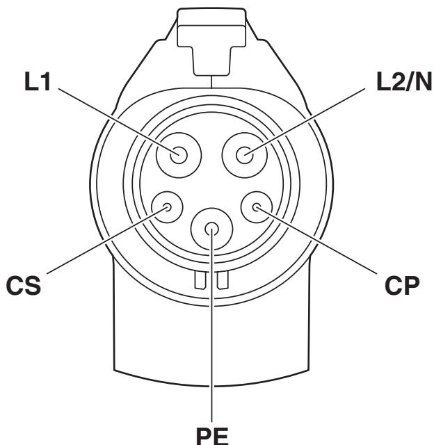
Pin assignment of the Vehicle Connector
