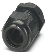
Cable gland, material for screw connection: PA, external cable diameter 11 mm .. 17 mm, shielding: no, connecting thread: M25 x 1.5, color: jet black RAL 9005
