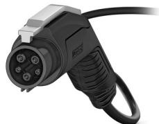
CHARX connect comfort, AC charging cable, with vehicle charging connector and open cable end, for charging electric vehicles (EV) with alternating current (AC) via type 1 vehicle charging inlets, without protective cap, Type 1, SAE J1772, 48 A / 250 V (AC), Without logo, cable: 18 ft, black, straight
