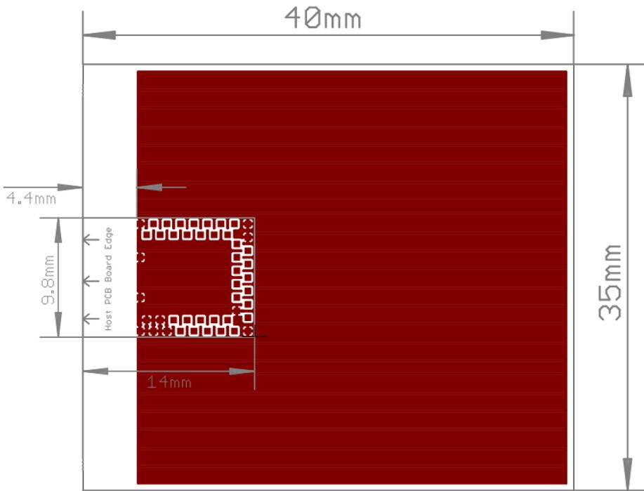
Figure 8: Recommended RF layout and ground plane
