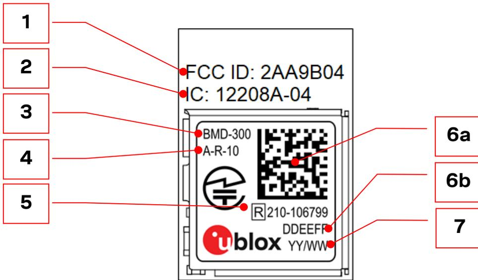
Figure 6: Module marking for type numbers BMD-300-A-R-10 and BMD-300-A-R-20
