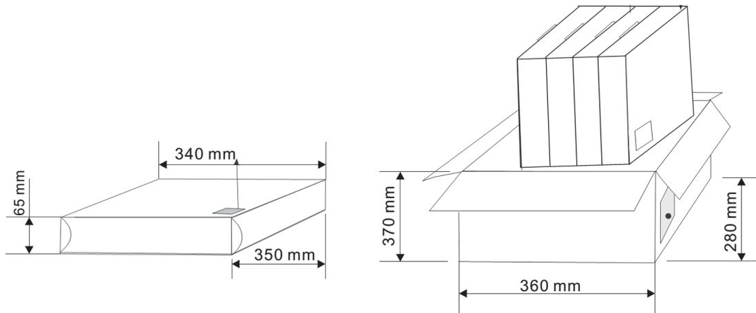
Figure 13: Reel cartons used for type number BMD-300-A-R-00
