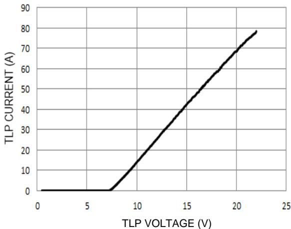
Figure 5 Pin1 to Pin2 TLP Curve ( $t_p = 100\text{ns}$ )
