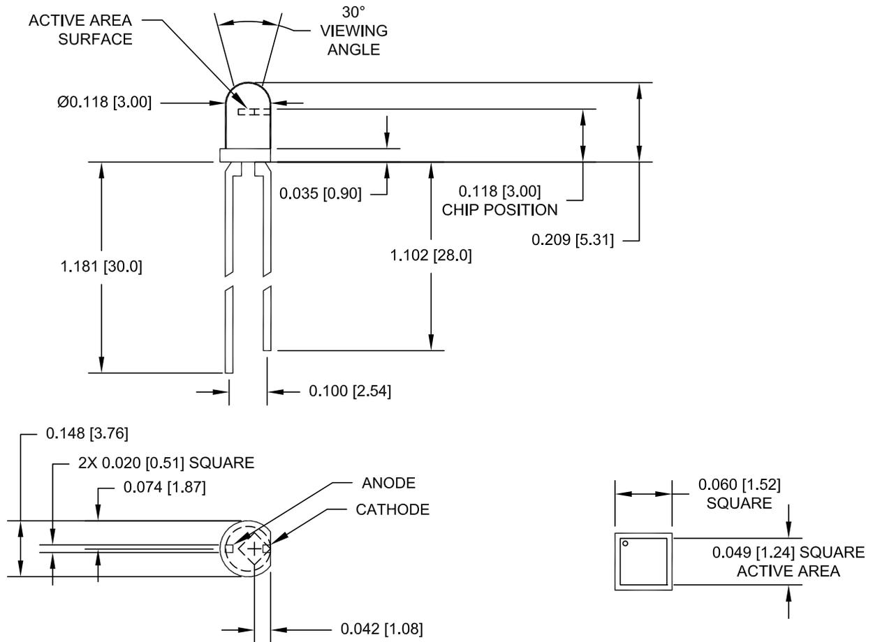
Soldering Conditions: 260°C 1/16 inch away from case for 3 seconds max.
