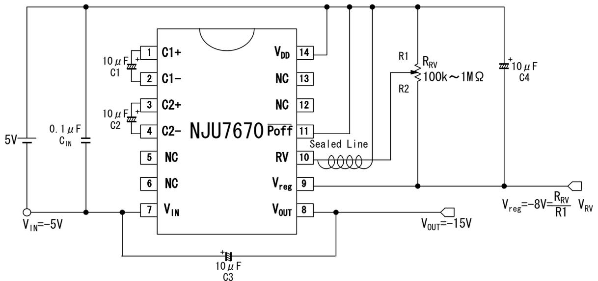
The IC may have a possibility not to operate properly with unstable supply voltage due to large transient current when the capacitor is charged or discharged.
