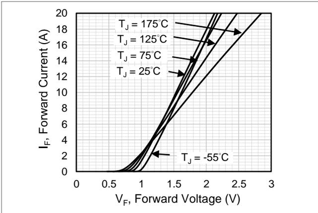
Fig.1 Forward Characteristics
