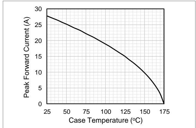
Fig.4 Current Derating Curve
