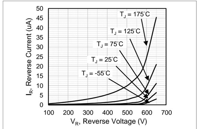
Fig.2 Reverse Characteristics
