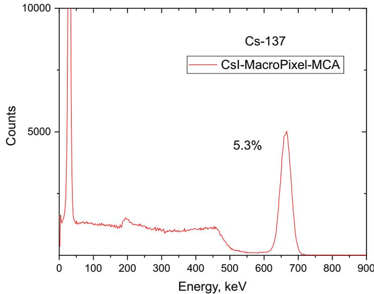
CsI(Tl) inorganic scintillation crystals have moderate light output of 55,000 photons/MeV, primary decay time about 1000 ns, reasonable density of 4.51 g/cc, and peak emission wavelength about 550 nm. Cesium Iodide scintillators are only mildly hygroscopic and do not easily crack under stress. Energy resolution of CsI-MacroPixel-MCA is typically near 6% at 662 keV.
