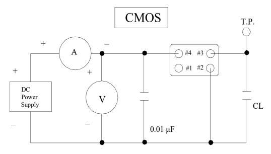
\*\*\*Because SMA series has no by pass capacitor. So,we recommend our customer to use capacitor 0.01  $\mu F$  in join Vcc and GND.
