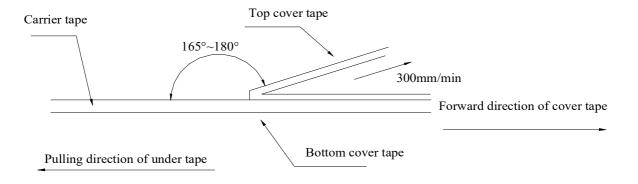
\*\*\* In the case, the cover tape is pulled off under the above conditions the cover tape adhesion strength should be as follows. \*\*\* Plastic tape:10.2g~71.4g
