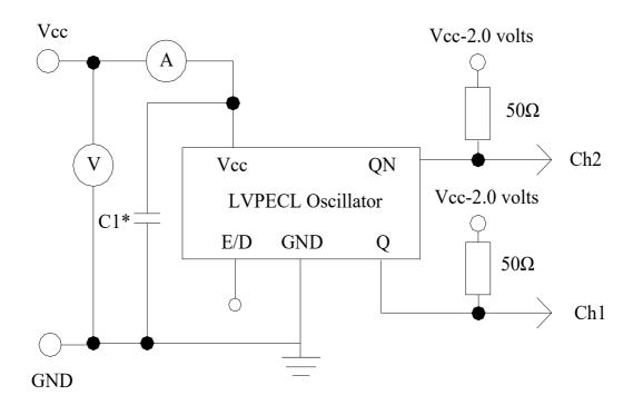
\*C1: A 0.01  $\mu F$  or 0.1  $\mu F$  decoupling capacitor is recommended.
