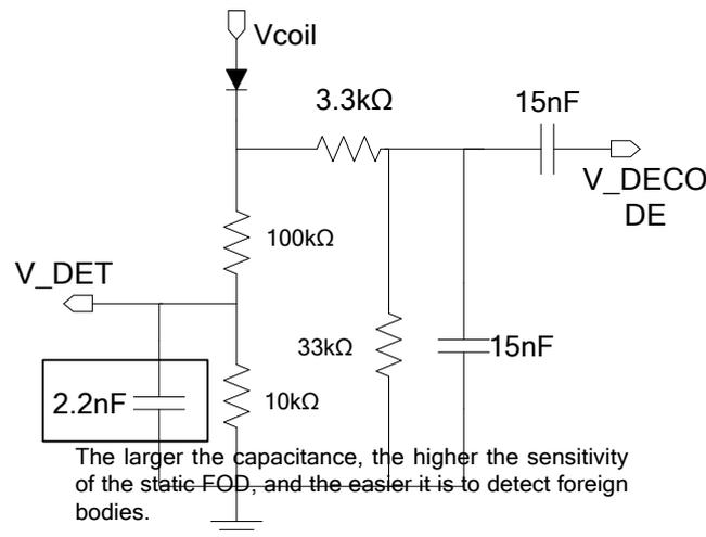
IP6806 can adjust the sensitivity of dynamic FOD by external resistor to GND on the LOSS\_THR pin; The LOSS\_THR pin defaults to a 100K resistor to ground, using standard dynamic FOD sensitivity; The larger the external resistor R\_Loss of LOSS\_THR, the lower the sensitivity of dynamic FOD, the less easy to detect FOD; The sensitivity of the dynamic FOD is set only by detecting the resistance of the LOSS\_THR pin at power-on;  $50K < R_{Loss} \text{ resistor} < 130K$ .
