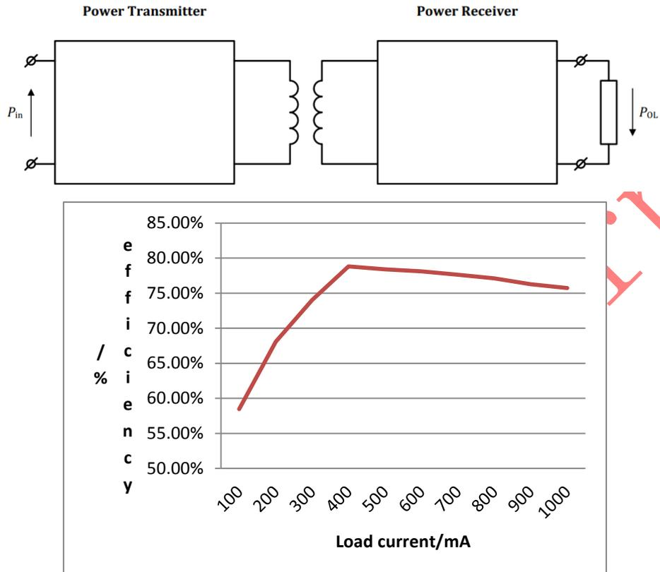
Figure System efficiency (using bq51020 RX)
