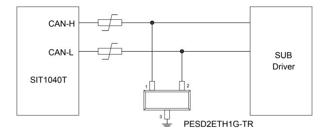
Typical Interface Application of CAN Bus Protection
