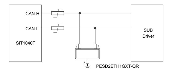
Typical Interface Application of CAN Bus Protection
