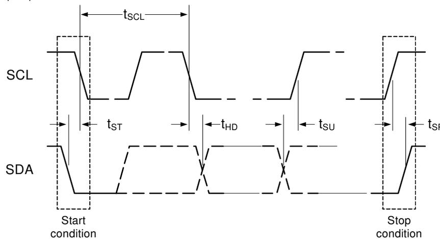
**Figure 2: I<sup>2</sup>C Data Transfer**
