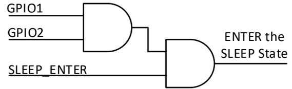
Figure 1. SLEEP State Entry Logic with SLEEP\_MODE I<sup>2</sup>C Bit = 0 (AND mode)
