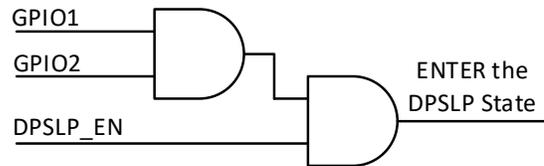
Figure 4. Always-On Configuration - DPSLP State Entry Logic with DPSLP\_MODE I<sup>2</sup>C Bit = 0
