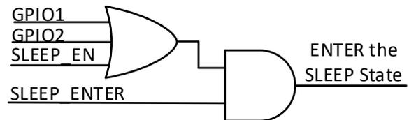
Figure 2. SLEEP State Entry Logic with SLEEP\_MODE I<sup>2</sup>C Bit = 1 (OR mode)
