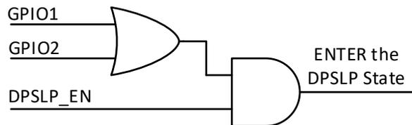
Figure 5. Always-On Configuration - DPSLP State Entry Logic with DPSLP\_MODE I<sup>2</sup>C Bit = 1
