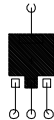
b. 95^\circ\text{C/W} when mounted on a 0.066\text{ in}^2 pad of 2oz Cu.
