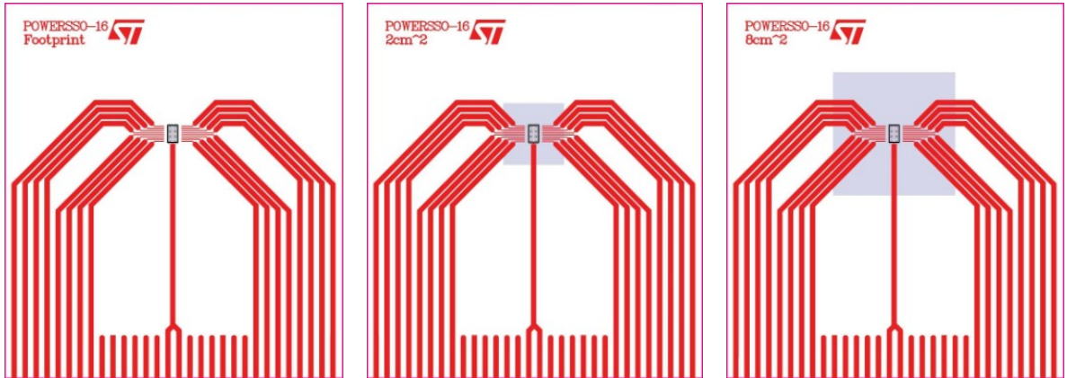
Figure 41. PowerSSO-16 on two-layer PCB (2s0p to JEDEC JESD 51-5)
