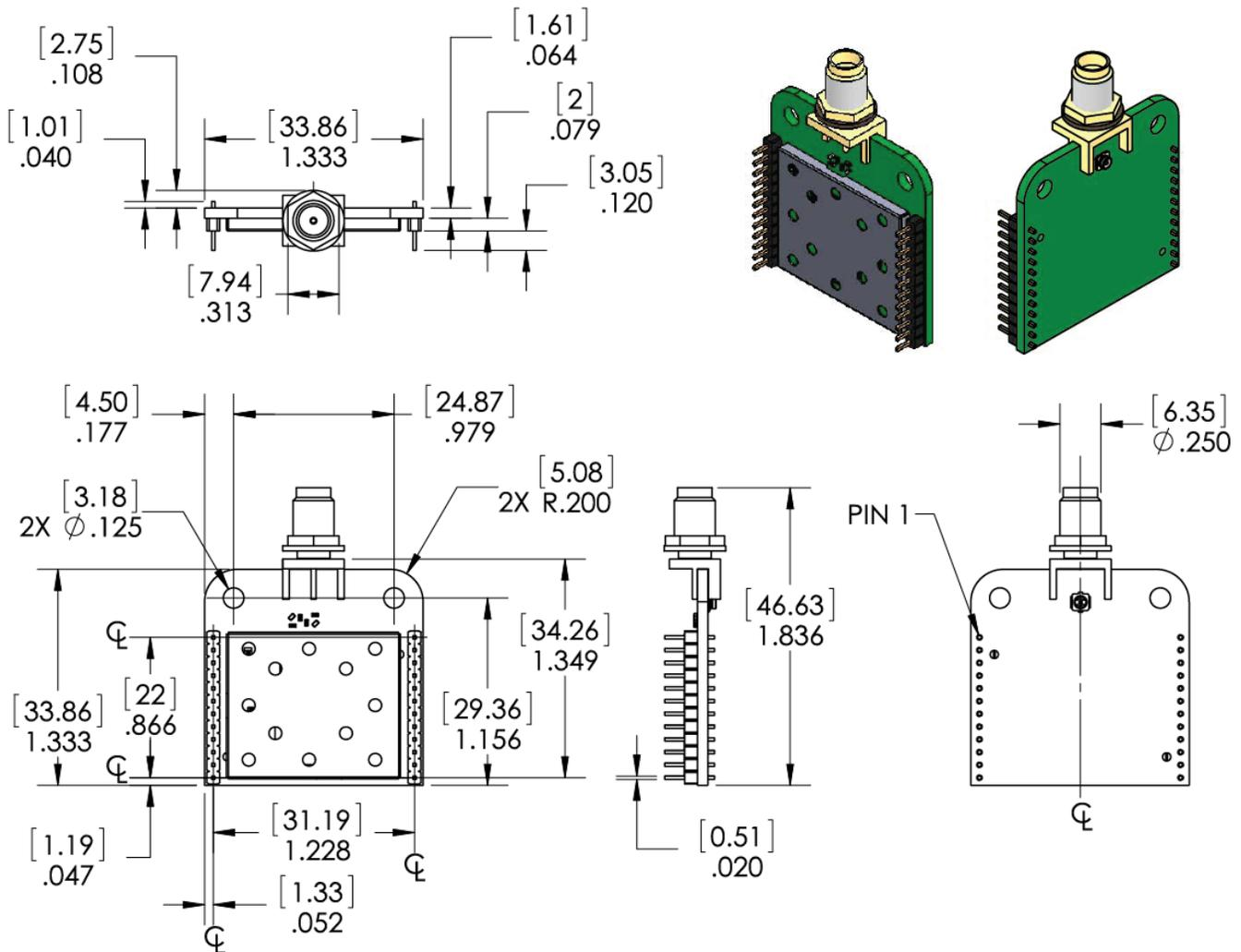
**Figure 1.1: RF220SUMechanical Drawing**
