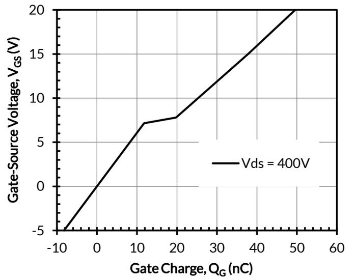
Figure 8. Typical gate charge at  $I_D = 20A$
