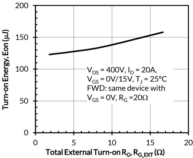
Figure 21. Clamped inductive switching turn-on energy vs.  $R_{G,EXT\_ON}$
